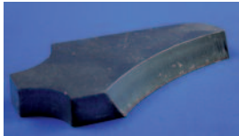
TRUMPF 5kW Mild steel 16t bevel
