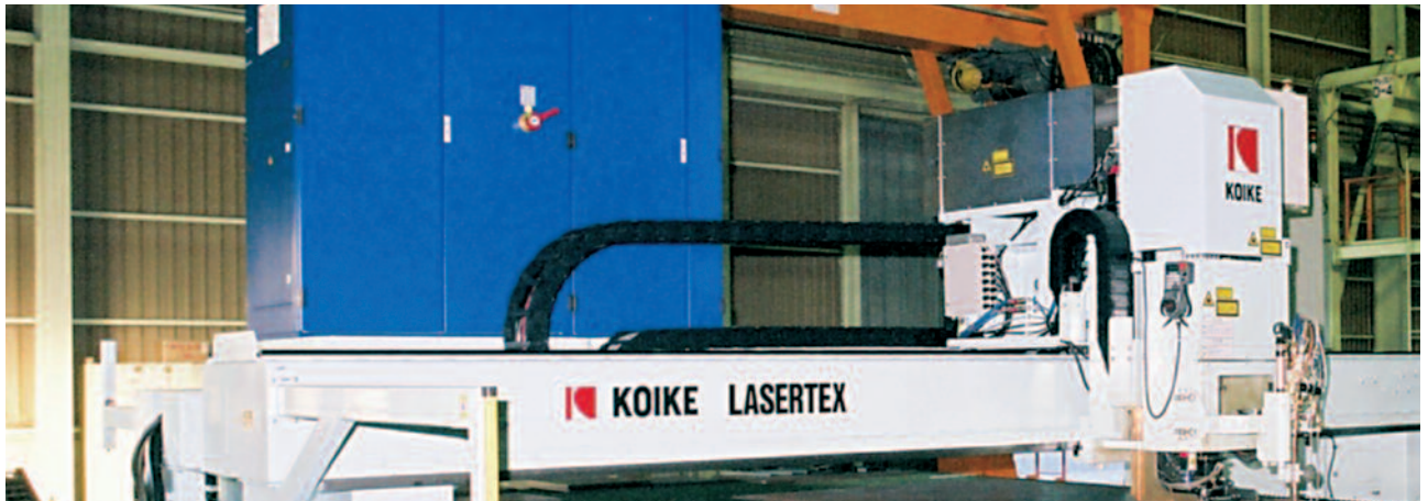
The TRUMPF resonator mounted on the carriage of a model LASERTEX-60TR Z series
