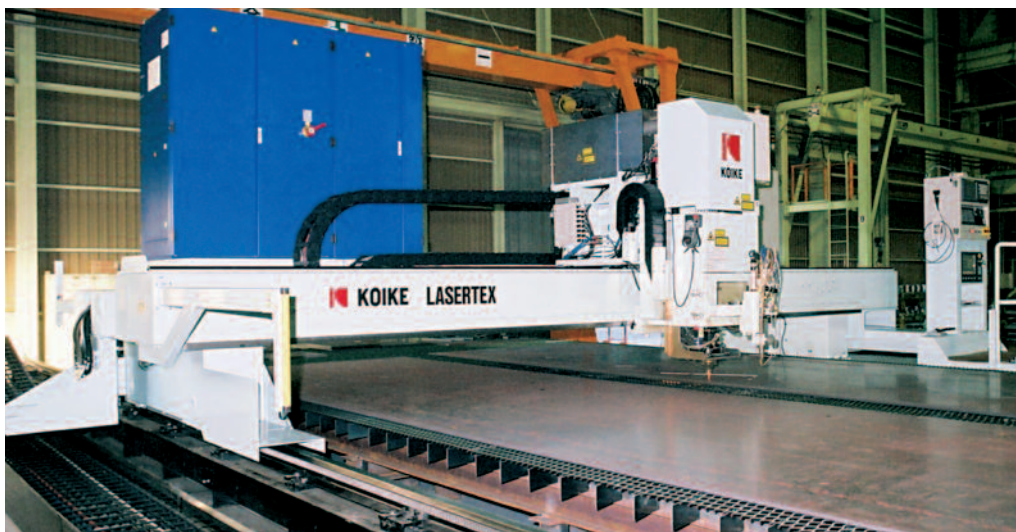
The TRUMPF resonator mounted on the carriage of the model LASERTEX-60TR Zseries
