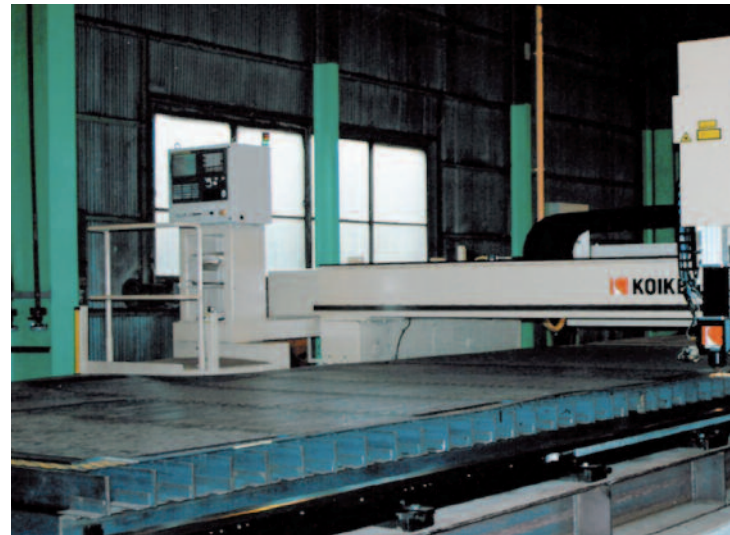
The FANUC resonator mounted on the carriage of the model LASERTEX-20 Zseries
