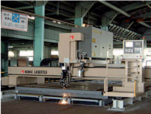
Mounting FANUC resonator on the carriage model LASERTEX-40 Z series
