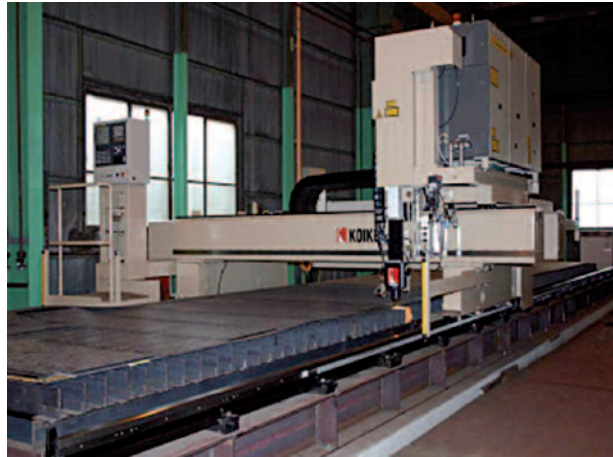
The FANUC resonator that is mounted on the carriage of a model LASERTEX-20 Z series
