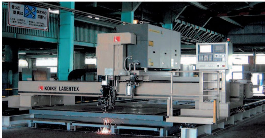
The FANUC resonator mounted on the carriage of the model LASERTEX-40 Z series
