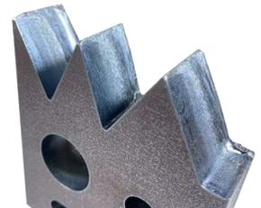
12kW Fiber Laser Cutting Material: SN490C 25mm
