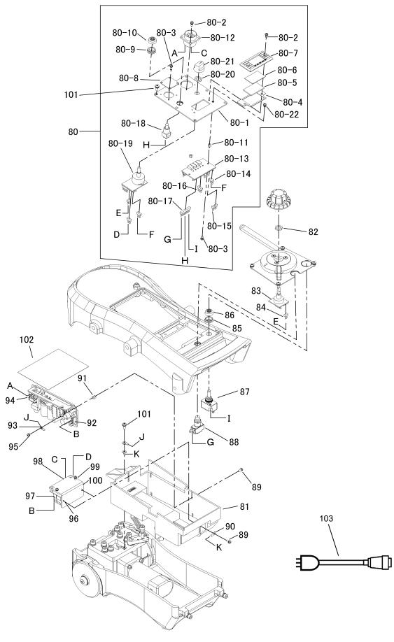
Electrical parts (TDK Lambda produces power supply)
