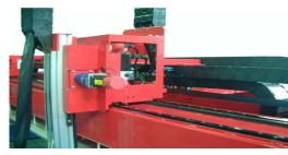
High speed accurate plasma cutting and line marking have become reality by adding linear guide ways and slides to the X-direction main drive carriage and sub carriage.
