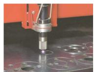
A vertical cutting within  $\pm 1.5$  degrees is obtained by using SUPER series. The upper edge of cut surface does not have roundness compared with any other plasma system.
