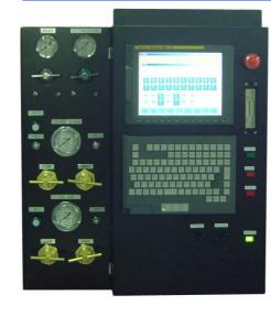
Centralized control station groups all control and operating functions in a single location, convenient to the operator.
