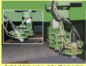
Control of torch posture of the 3D-Link system makes the torch-height control point on the cut material a center point and executed.
