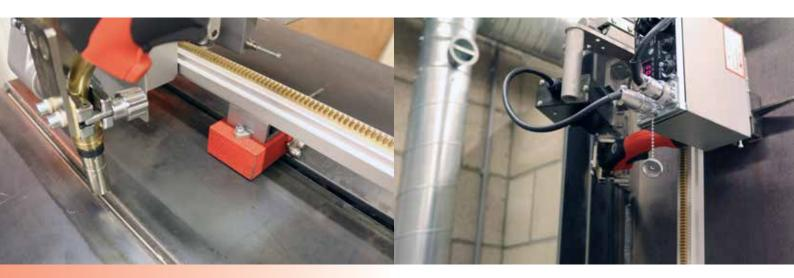
The IK-72W series is used for straight welding in horizontal and vertical positions using 1 dimensional rail and curved and twisted plane welding using 2 and 3 dimensional rails. By using same rail system as the cutting machine IK-72T, cutting and welding can be done with IK-72 system in convenient and lightweight package.
