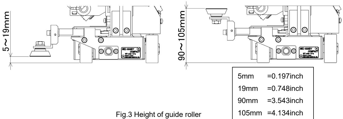
Fig.3 Height of guide roller
