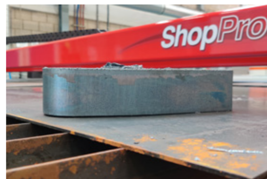
Up to 50mm cutting thickness (oxyfuel)
